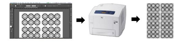
Figure 3-2 The printing process of paper-based device using a wax printer.
