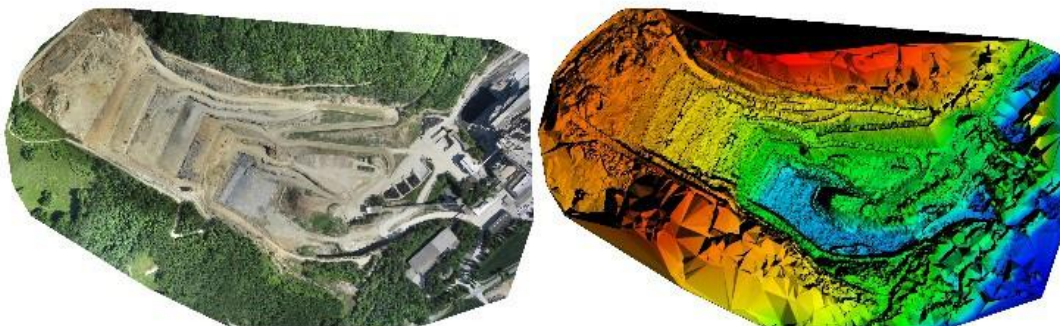
Figure 1: Orthomosaic and the corresponding sparse Digital Surface Model (DSM) before densification.
